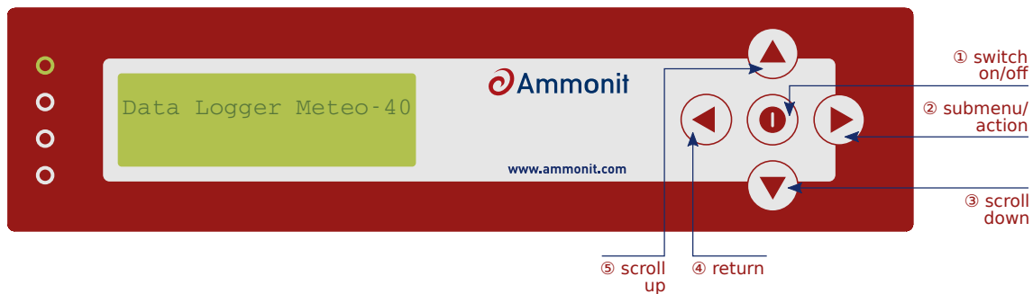
Figure 9.1: Use of the Meteo-40 buttons
